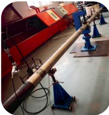
▲ 整机检测验收 Tool assembly test and inspection
